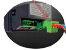
3. Voltage Output to power the next meters (up to 16)
