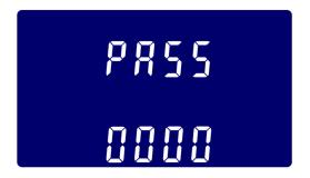
Setting up is password-protected so you must enter the correct password (default '1000') before processing. If an incorrect password is entered, the display will show: PASS Err
