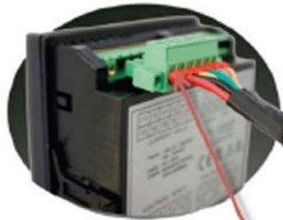
1. Current Transformer Input
