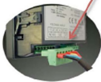
2. Fuse Voltage input
