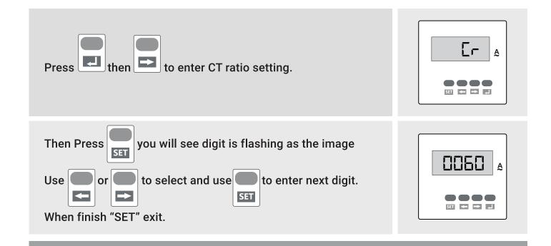
The Range is from  $0001 \sim 9999$ . For example: if set the ratio to be 60, That means the Primary Current is Secondary Current x 60 = 300A.
