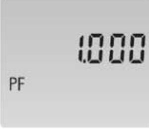
A digital display showing the number 1.000 in large black digits. Below it, the unit 'PF' is displayed in smaller letters. At the bottom left, there are three small vertical bars.  | Power factor<br>Example: 1.000     |
