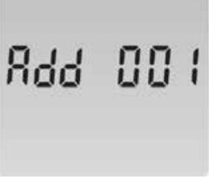
A digital display showing the word 'Add' followed by the number 001 in large black digits. At the bottom left, there are three small vertical bars.                                 | Modbus Address<br>Example: 001     |
