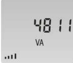
A digital display showing the number 4811 in large black digits. Below it, the unit 'VA' is displayed in smaller letters. At the bottom left, there are three small vertical bars.    | Apparent power<br>Example: 4811VA  |
