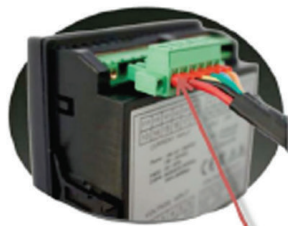
1.Current Transformer Input
