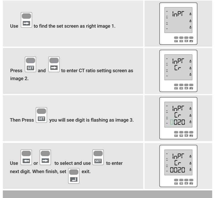
The Range is from  $0001 \sim 9999$ . For example: if set the ratio to be 20, That means the primary current is secondary current 5x20 = 100A.
