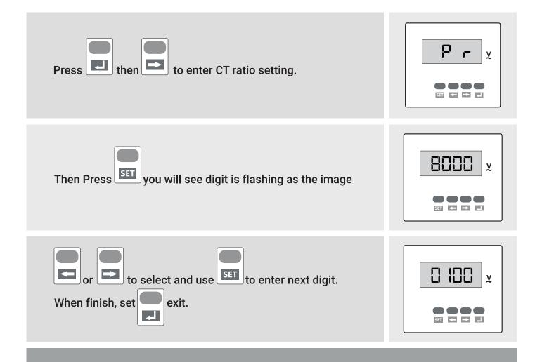
The Range is from  $0001 \sim 9999$ . For example: if set the ratio to be 100, that means the primary voltage is secondary voltage x 100.
