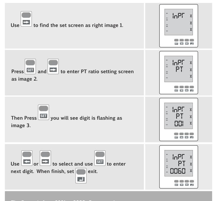
The Range is from 0001 ~ 9999. For example: if set the ratio to be 60, That means the Primary Voltage is Secondary Voltage x60.
